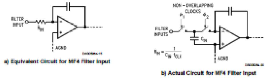
a) Equivalent Circuit for MF4 Filter Input
